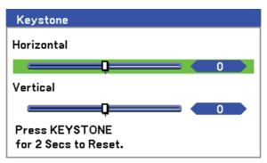
Select Horizontal or Vertical using ▲or▼ then, use ◀or▶ to adjust the projected image appearance as required.
